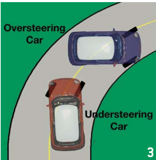
Understeering is when the car continues to plow forward even when the front wheels are turned into the turn because the car is set up to keep more weight on the rear wheels than on the front wheels. Oversteering is when the car's rear end rotates around the front wheels in a turn because the car has more weight on the front wheels than on the back wheels. Because oversteering is more dangerous than understeering, most cars are set up by their manufacturers to understeer.
