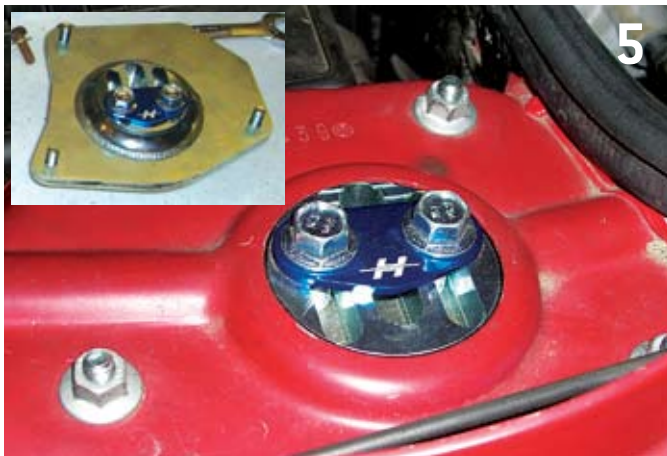
Hotchkis Camber Plate: The MINI suspension comes with too little negative camber in front. Fixed or adjustable camber plates can address this. These Hotchkis plates don't affect ride height, and can give up to four degrees of negative camber if the right springs are used. Improving the front camber will decrease understeer, improve turn in and in my case, has increased tire life.
