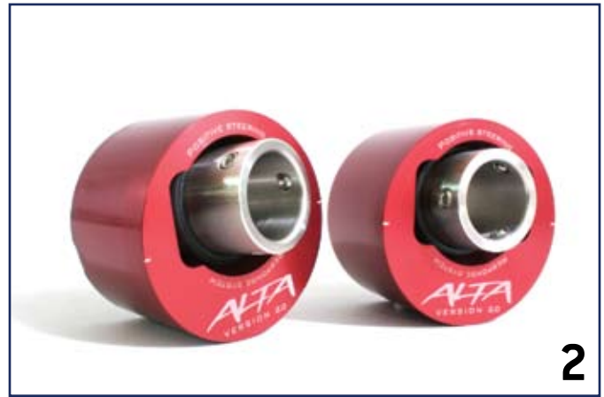
Alta PSRS: This is a front control arm rear bushing replacement. Besides reducing compliance over the stock rubber, it allows for slight geometry modification as well, increasing caster for improved steering return to center.
