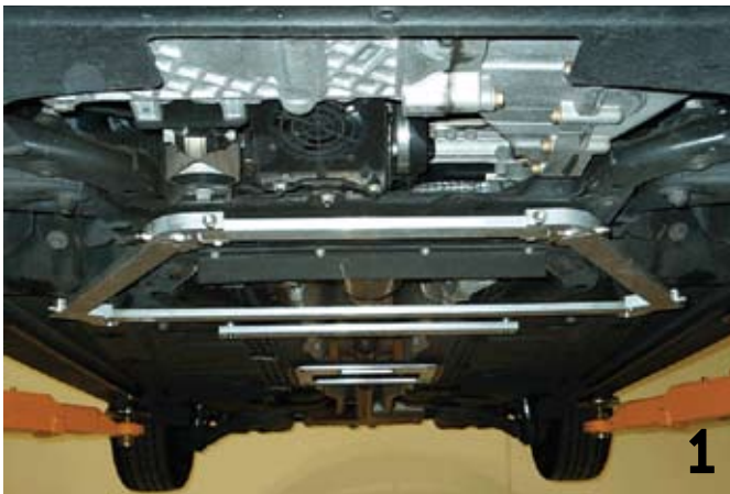
M7 Under Strut System: The suspension can only do its job if the geometry is fixed. Stiffening aids, like this chassis brace system, up to and including a full cage, make the car much more rigid. This is especially an area of concern for convertibles, that don't have the top to form a full boxed shape.
