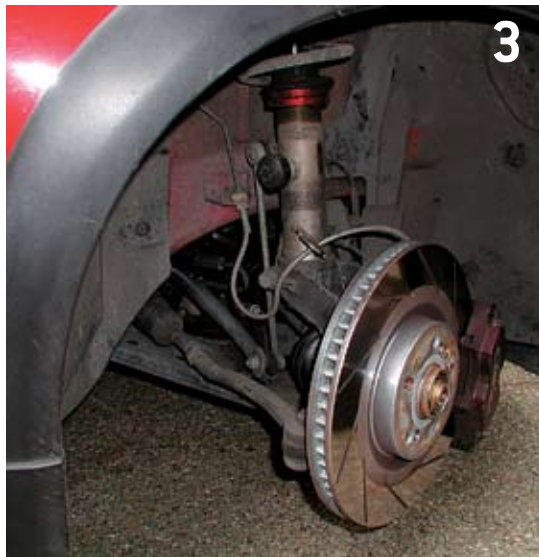
Figure 3, near right, is a picture of the front suspension, with the Macpherson Strut connecting the wheel at the top, and an a-arm connecting it at the bottom. Far right, figure 4 shows the rear suspension from the side. It is easy to see why this is called a "trailing arm" suspension.
