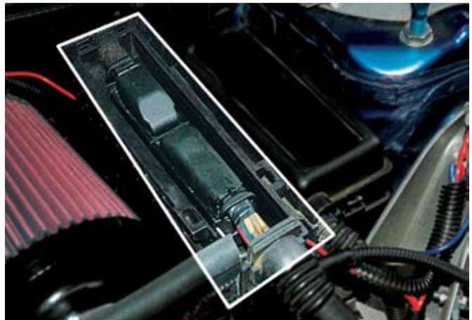
The ECU exposed: The ECU is next to the air intake. With the cover removed, the wires going into the engine compartment can be seen at the front, and the connector into the passenger compartment at the rear. The computer itself is just below the connectors.
