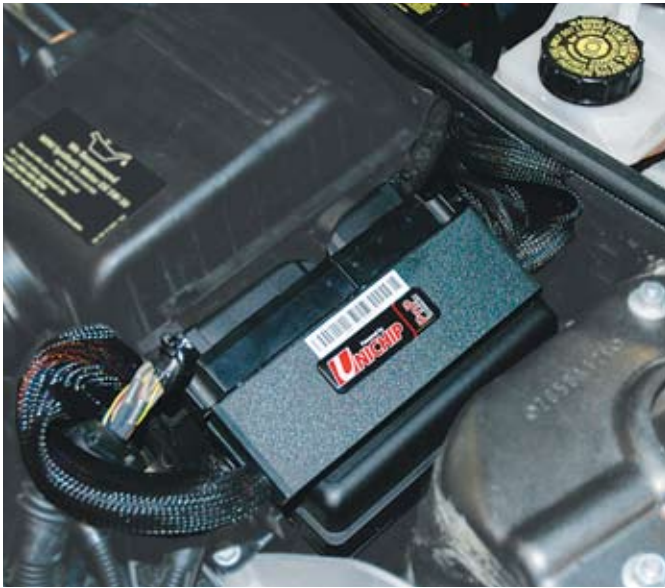
Piggy-back units, such as that made by UniChip, are named for obvious reasons, and are connected between the engine and the ECU.
