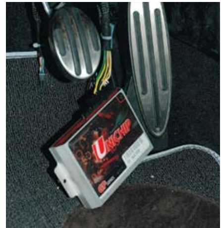
The system easily plugs in to the car’s wiring harness and ECU, with the computer inside the driver wheelwell under the dash. Dynamometer runs showed the immediate contribution of the system.
