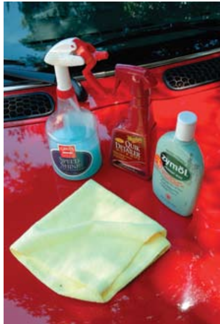
Stage 2: Keep the Shine Looking Good. Once every few weeks, or whenever you want the car to look its best, use an instant detailer applied and removed with a microfiber cloth. If you want a little extra, use a one-step polish/wax.
