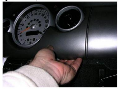
IMPORTANT: On newer '05 and '06 MINIs you don't need to do this step! Instead you will find that once the Torx screws are removed, you can slightly drop the downtubes so that they can be lifted out from behind this trim panel – you can't remove them but you can push them sideways sufficiently to access the screws holding the toggle switch panel (see next step).
