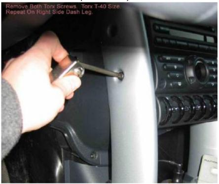
Accessing the top Torx screw where a glovebox or knee bolster is present will require opening the glovebox door or releasing the knee bolster. To release the knee bolster, grab the top edge with both hands. Pull down sharply keeping the pressure toward the direction of the door in order to prevent the bolster from scratching the downtube when it comes free. Once free it can be swung down out of the way to provide clearance to access the Torx screw.
