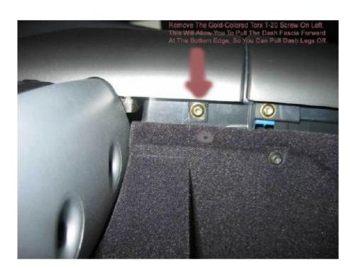
9) Provide clearance: Pop the lower clips of the fascia by grabbing its lower edges and giving a medium sharp tug. Pull the fascia outward just far enough for the tops of the downtubes to clear.
