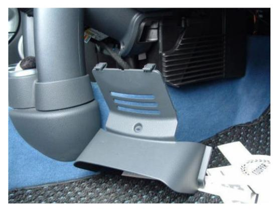
Next you need to reach up behind the toggle switch panel, and feel for the connector - you can follow the wire bundle to find it. The original connector is latched into the back of the toggle switch panel; a retaining bump on the back of the connector must be pushed down to allow a latching clip to be slid over it; this will release the connector from the toggle switch panel:
