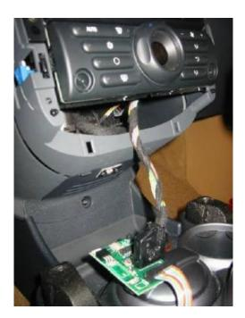
This pic from Bill shows the MINI circuit pushed in behind where the toggle switch panel normally fits, with the harness from it going to the toggle switch panel (the downtubes are still removed)
