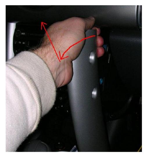
At this point you can remove the Torx screws holding the toggle switch panel, and pull it out to access the connector behind. Remember to install the circuit through the lower trim piece – there is not room to slide the circuit through the opening behind the toggle switch panel once the original connector is plugged onto it.
