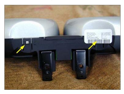
Release the tabs by using a flat screwdriver to lift the black tab over the white tab, while pulling the back cover away from the gauge.
