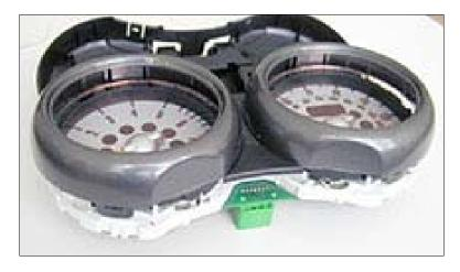
Snap the trim ring onto the gauge, and ensure that all 4 tabs engage completely. Verify that the odometer reset button moves freely when pressed; if not, readjust alignment of the speedometer lens.
