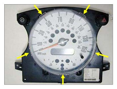
To remove, press down firmly on the two tabs at the top. The tabs will release and the lens can be pulled away from the gauge.
