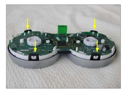
Note: If you have chrome rings, the black middle trim piece may be attached underneath with double stick foam tape. If there is tape, you'll need to separate the pieces far enough apart that you can insert something to pry or cut the double stick tape. Dental floss works well for cutting through the tape.
