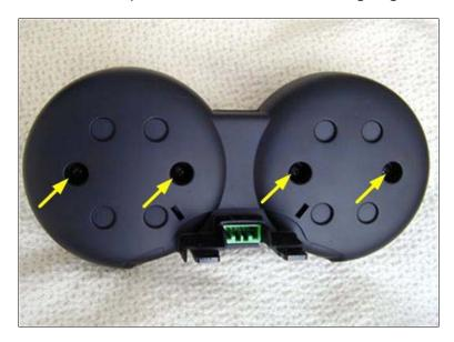
Unclip the two bottom tabs of the back cover. If one of the tabs is covered by a label, cut or remove it to expose the tab.
