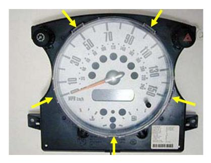
The lens does not pop off easily unless you press at least 3 of the points simultaneously. We suggest using thumb and forefinger of both hands to press in simultaneously at the upper 4 points.
