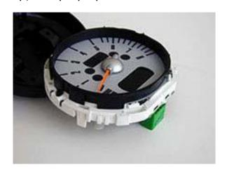
Place the new lens on top of the black ring, with the cutout at bottom.
