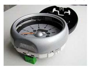
Snap the trim ring onto the gauge, and ensure that all 3 tabs engage completely.
