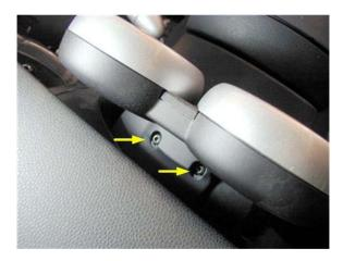
Pull the gauge straight back away from the dash. The gauge will become free (but still attached to the wiring harness).
