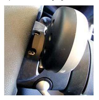
Pull the gauge straight back away from the dash. The gauge will become free (but still attached to the wiring harness).
