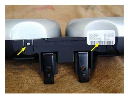
Release the tabs by lifting the black tab over the white tab, while pulling the back cover away from the gauge. Separate the back cover from the gauge.
