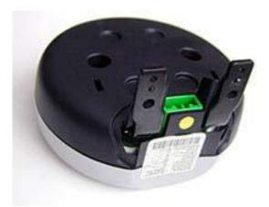
Release the tab by lifting the black tab over the white tab, while pulling the back cover away from the gauge. Separate the back cover from the gauge.
