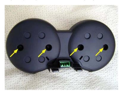
Unclip the two bottom tabs of the back cover. If one of the tabs is covered by a label, cut or remove it to expose the tab.
